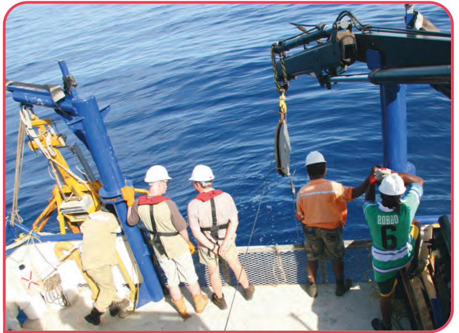
Lowering a sediment corer to collect seabed samples off PNG.
