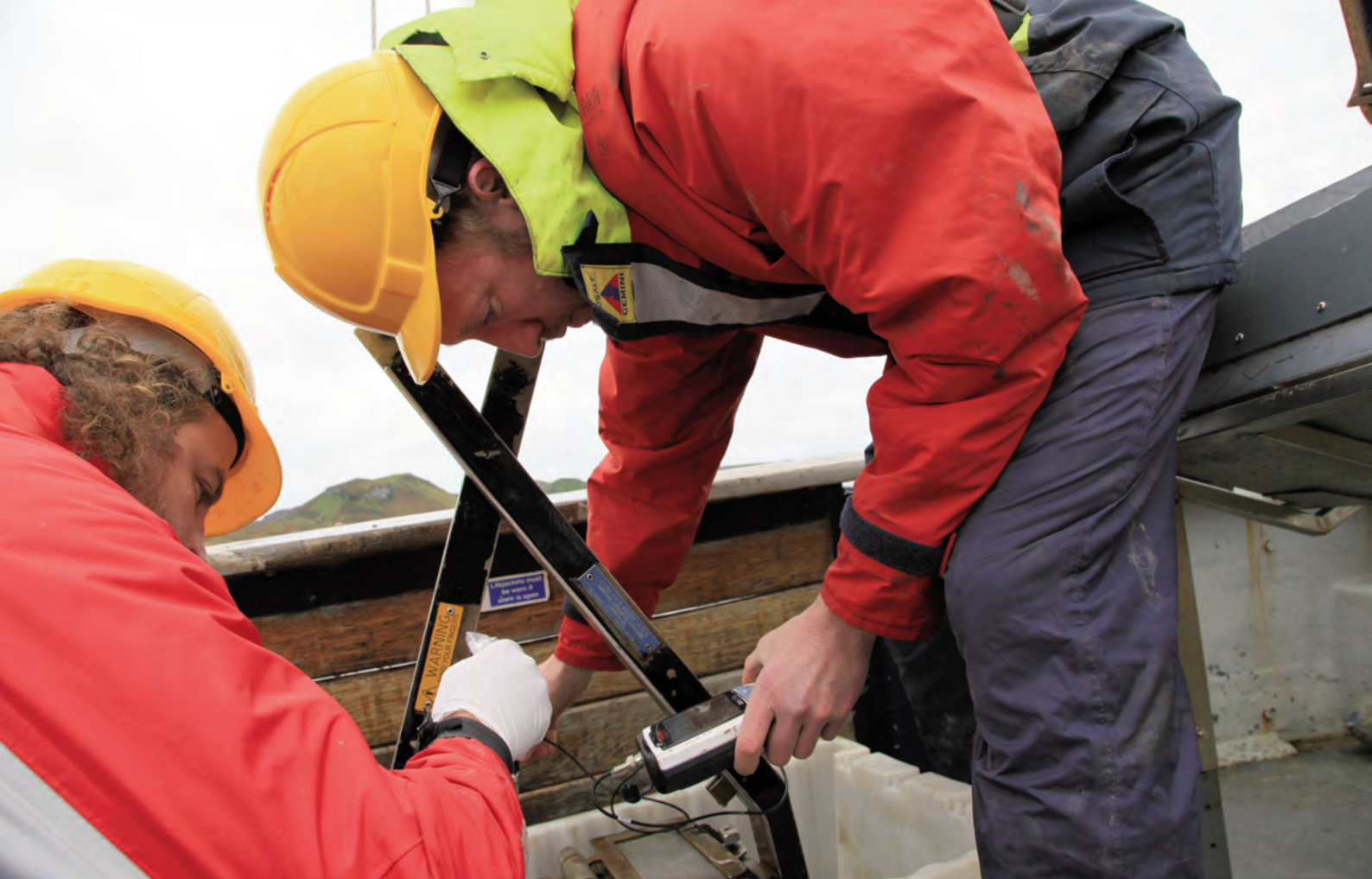
Fig. 1: Simultaneously taking a sample for 'metagenomics' analysis and measuring sediment oxygenation status (redox) in a grab sample taken from around a fish-cage. We found that measured DNA diversity was highly correlated with redox and may offer a viable approach to benthic monitoring.
