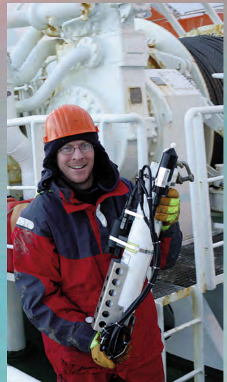
Finlo pictured holding a moored CTD unit - an instrument used on the Arctic Observatories.
