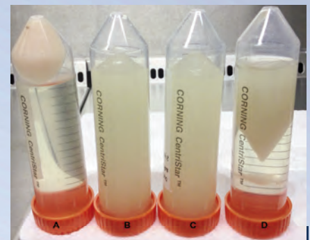
Fig 3. Optimising gum production by the marine bacterium DG1864 (picture courtesy of Dr Mariana Fazenda, Univ. Strathclyde). A, no glucose; B-D, glucose plus growth at different temperatures).
